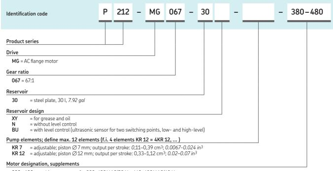
380 - 480 = multi-range motor for 380 - 420 V AC/50 Hz, 440 - 480 V AC/60 Hz
