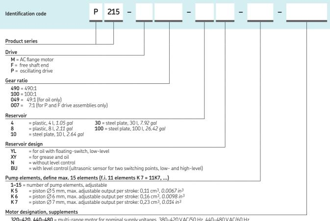
320-420, 440-480 = multi-range motor for nominal supply voltages, 380-420 V AC/50 Hz, 440-480 V AC/60 Hz
