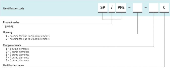
C = actual version for  $p_{max}$  4 000 bar, (58 000 psi), rotary-operated, double-sided drive shaft, ratio 1:1
